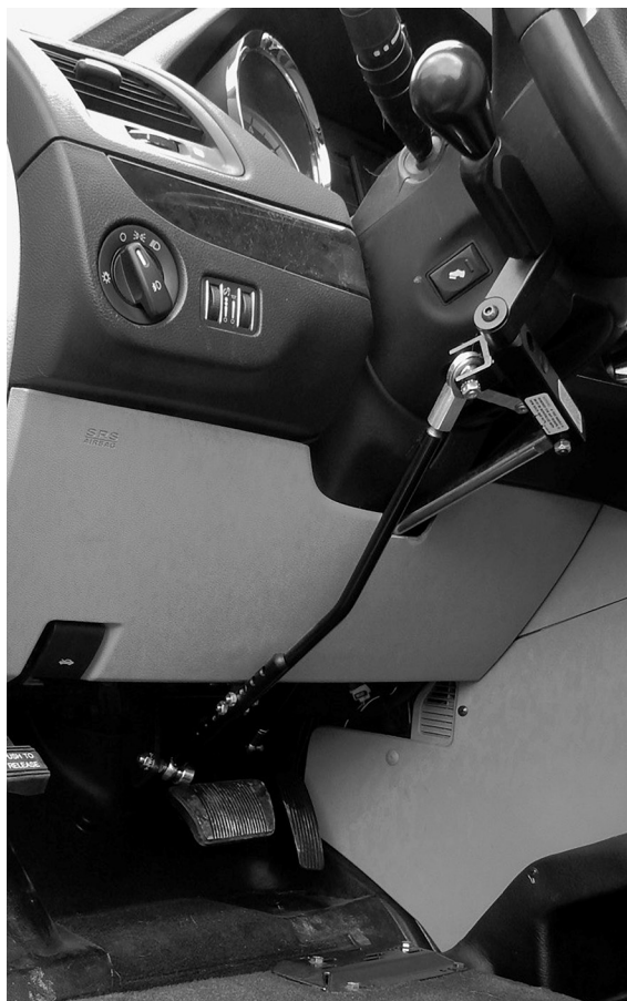
To operate the hand controls, a lever is pushed forward to engage the brake and down for the accelerator.
