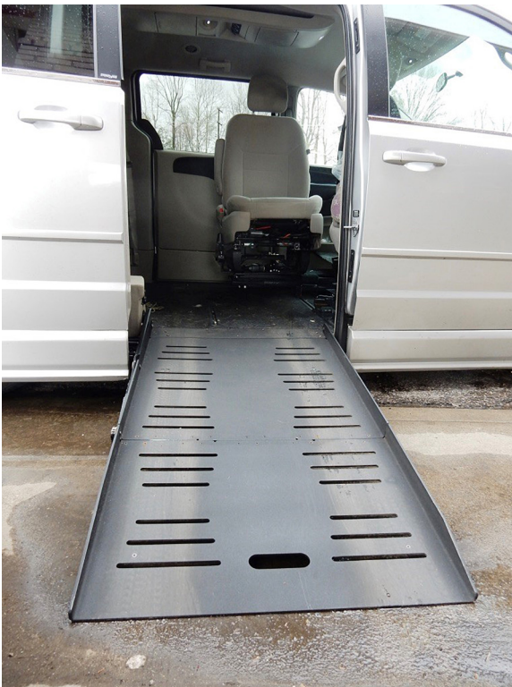
Minivan with folding ramp extended. The driver's seat is turned so that I can transfer into it from my chair.
